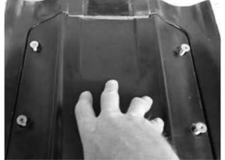
When installing the ride plate bolts, loosely install each bolt while pushing up with the ride plate so it sits flat with the mounting points. Then tight each, front first, then back two. If your ski uses 6mm bolt, please beware you can over tighten the bolt past the Flex material. Use loctite and silicone on final install.
